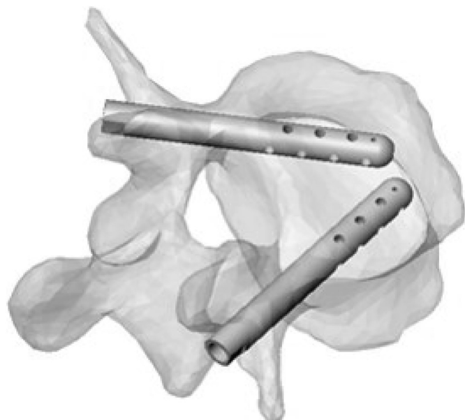
Fig. 1. Schematic view of V-STRUT ® before cement injection.
